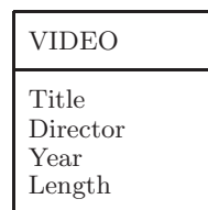
Figure 3.53: An entity class such as VIDEO has several attributes. (example from MS Access)
