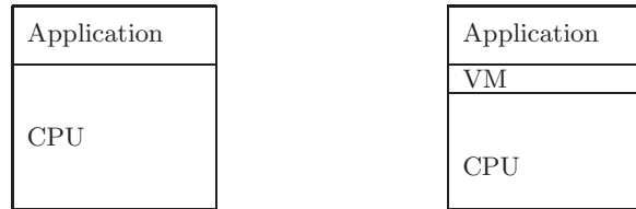
Figure 7.42: Virtual machines help to separate software from hardware dependencies. (hand drawing)
