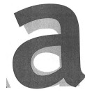
Figure 10.7: Fonts can improve readability. Clearfont font (dark "a") has recently been developed to improve the readability of highway signs compared to the older font (light "a").
