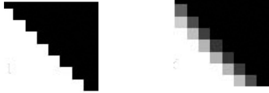
Figure A.148: Rather, than a sharp edge, pixels in a display create a jagged edge (left). To create the appearance of a smoother edge, the edge pixels are grayed out.
