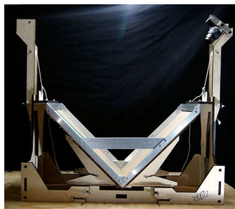
Figure 10.8: This book scanner is designed so the page images can be captured without breaking the spine of the book. (check permission)
