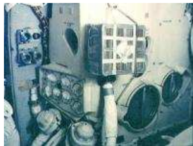
Figure 3.44: “Houston, We’ve Had a Problem”. After the Apollo 13 accident, the oxygen supply for the crew was endangered. A canister was improvised to filter the air.
