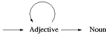
Figure A.37: State machine notation showing that one or more adjectives can be repeated before a noun.
