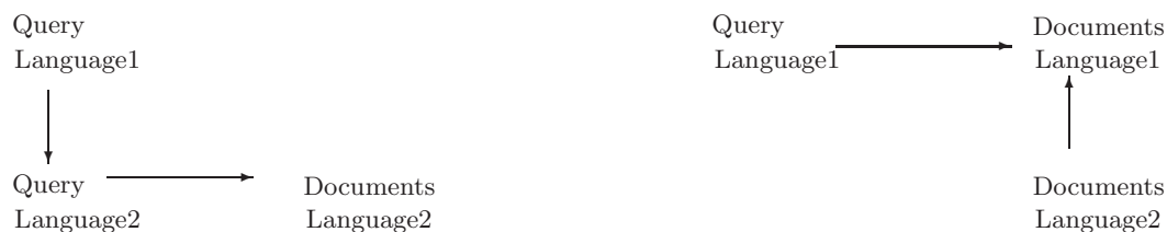
Figure 10.63: Two models for cross-language document retrieval. Translating the query or the document. It may be better to do both and combine the results from the two approaches.
