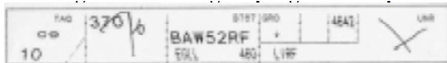
Figure 5.34: Shared information resources often provide support for distributed cognition. Here's a tracking slip user by air traffic controllers as a record for a flight. The highly structured slips provide a quick overview of the flight and can be easily transferred across shift changes. Recognizing how they are used can be helpful for developing computerized air traffic control tools. (check permission)
