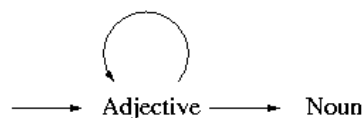
Figure 6.7: Grammars are closely related to state machines. Here a recursive state machine link shows that one or more adjectives can be repeated before a noun.
